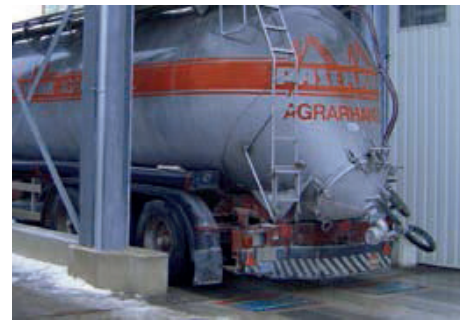
WWS installed flush floor, for dynamic weighing >>
